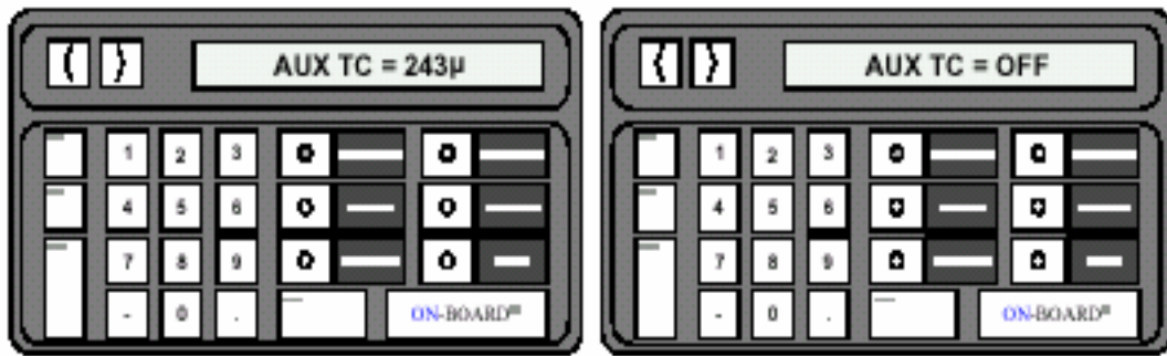
Figure 3-6: Auxiliary Thermocouple Gauge Pressure
