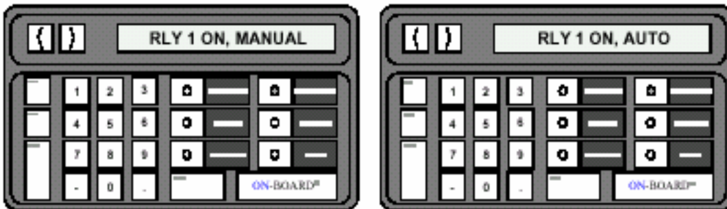
Figure 3-41: Relay 1 ON/OFF and Auto/Manual Control Display
